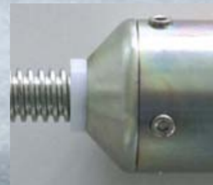
Back limit stop, here with polyamide ring
